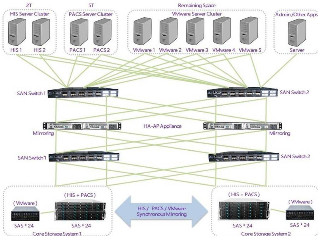
**Figure 3. HTCM Datacenter – Topology Diagram**
